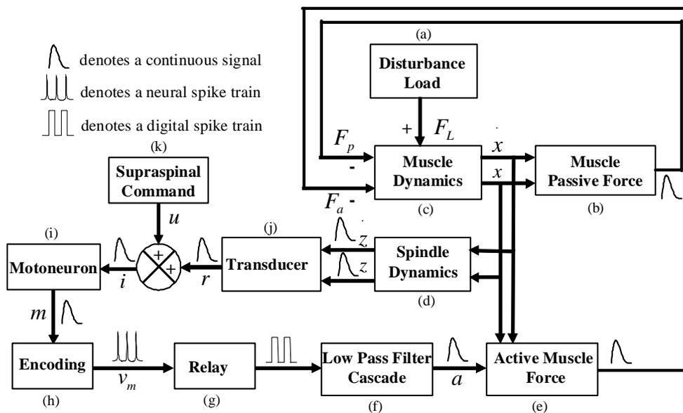
Figure 1: Block Diagram of Simulink Model
