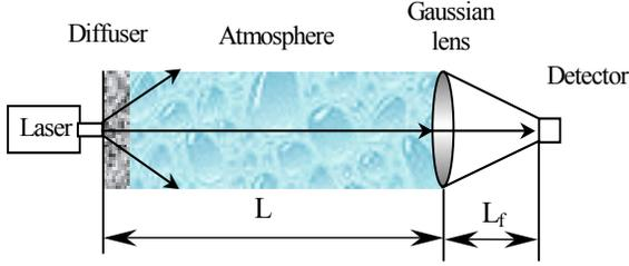
**Figure 1.** Propagation of partially coherent beam
