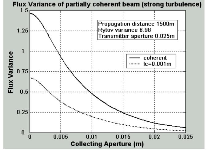
**Fig. 4** Flux variance  $\sigma_I^2(L + L_f, \Omega_G)$  as a function of the radius of the collecting lens  $W_G$  for coherent and partially coherent beams in strong turbulence.
