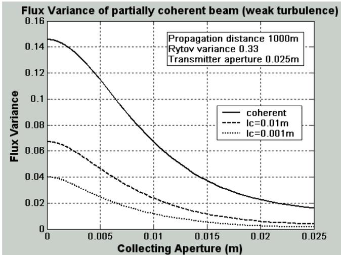
**Fig. 2** Flux variance  $\sigma_I^2(L+L_f, \Omega_G)$  as a function of the radius of the collecting lens  $W_G$  for coherent and partially coherent beams in weak turbulence.
