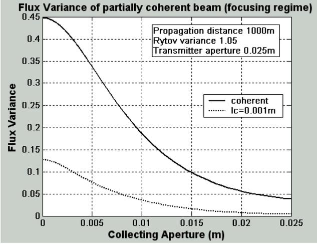
**Fig. 3** Flux variance  $\sigma_I^2(L + L_f, \Omega_G)$  as a function of the radius of the collecting lens  $W_G$  for coherent and partially coherent beams in focusing regime .
