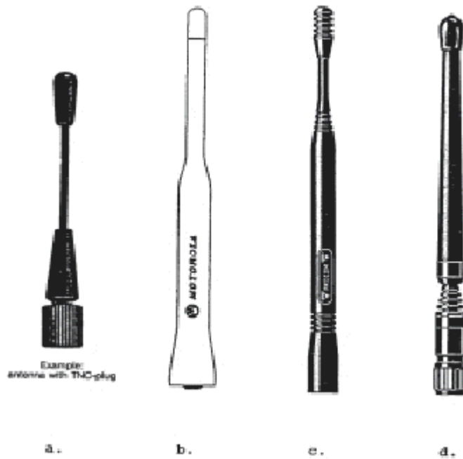
Examples of whip antennas for 900 MHz. a) \lambda/4 antenna, height point, height 210 mm, d) Top fed \lambda/2 antenna, height 200 mm 100 mm, b) 3\lambda/8 antenna, height 150 mm, c) \lambda/2 antenna with an elevated feed
